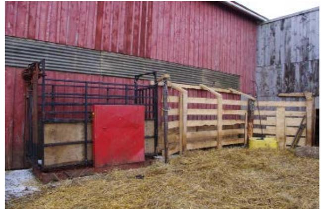
*Basic handling system with old scale mounded under chute with head gate*
